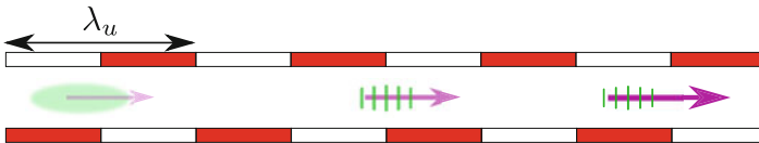
Fig. 3.3 Build-up of electron microbunches. During its passage through the undulator the electron bunch is split up into narrow electron microbunches that radiate coherently (adapted from [8])
